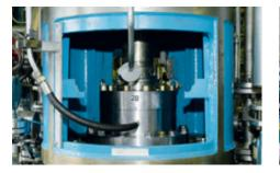
Wacker Chemie AG in Burghausen, Germany, seals a number of top-drive high pressure reactors for polymer dispersion manufacturing with **HSHLY-D** type high pressure seals with cooling flange. A shared buffer system supplies all the seals. Operating conditions:  $p_1 =$  vacuum ... 100 bar (1,450 PSI); t = ... 100 °C (212 °F); n = 25 ... 100 min<sup>-1</sup>.
