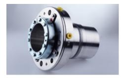
During the production of ammonia, carbon dioxide is removed from the process with Benfield solution – an aqueous potassium carbonate solution with diethanolamine. **HJS1** type mechanical seals have proven to be best for sealing the pumps in this area. Typical operating conditions:  $p = 2 \dots 4$  bar (29 ... 58 PSI);  $t = 100 \dots 150$  °C (212 ... 302 °F); n = 1,500 min<sup>-1</sup>.
