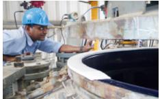
Tytan Organics Chemical Co. in the United Arab Emirates uses glass-lined reactor vessels to manufacture concrete plasticizers. The flanges and covers are sealed with **Burachem multi-gaskets** made from pure PTFE. Medium: Napthalene sulphonate formaldehyde. Operating conditions: p = 6 bar (87 PSI); t = 220 °C (428 °F).
